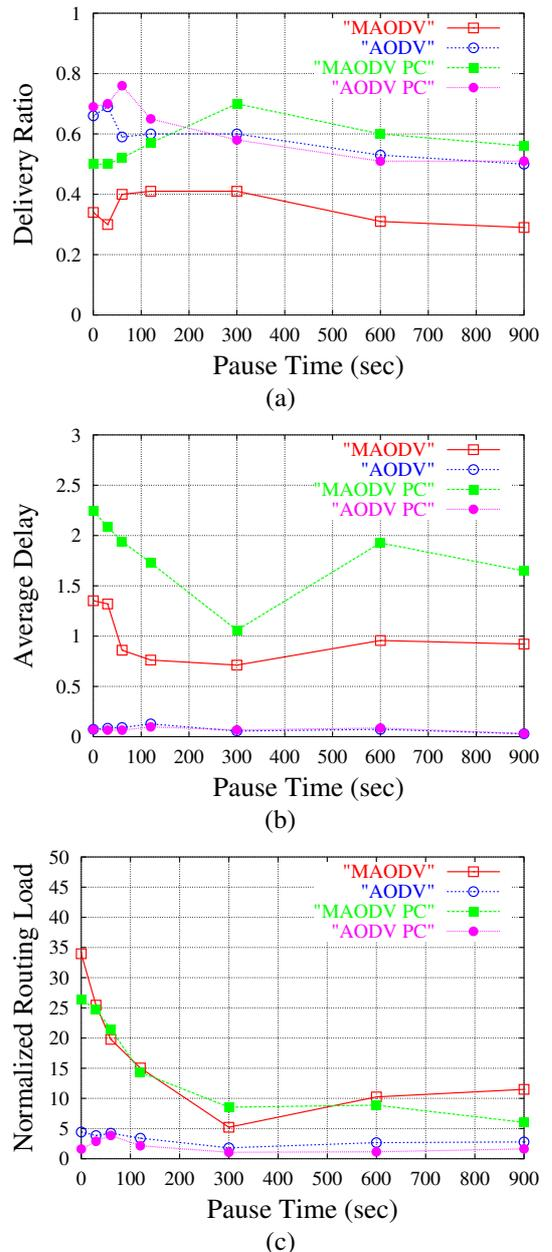
Fig. 2. (a) Delivery ratio, (b) average delay and (c) normalized routing load in a scenario with  $N = 50$  nodes, radio range equal to 250 m, packet generation rate  $\lambda = 4$  pck/s and 10 active source nodes.
